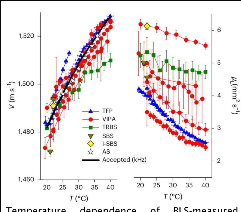
Temperature dependence of BLS-measured hypersonic speed (left) and kinematic longitudinal viscosity (right) of pure water obtained from different instruments and labs around the world. (Taken from Ref [1]).
